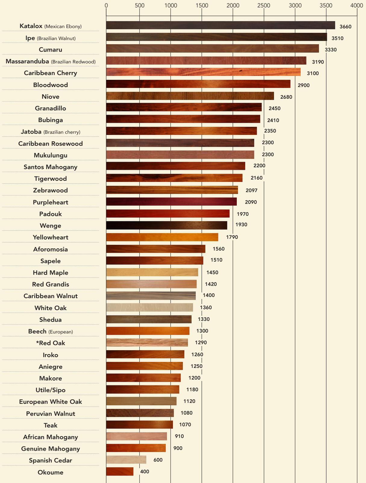
\*Red Oak with a Janka rating of 1290 is the industry benchmark for comparing the relative hardness of different wood species. The Janka hardness test provides a relative scale where the higher the number indicates the harder the wood.
